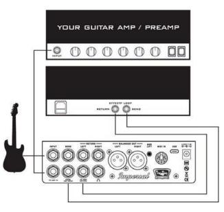
**IMPORTANT** - if placing the IMPERIAL preamp on top of a head cabinet or combo, you MUST place the IMPERIAL preamp on the opposite side of your amp's main transformer (usually the input side). Placing the IMPERIAL preamp over the mains transformer may cause noise to enter the signal chain.
