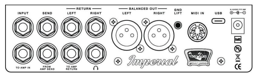
• INPUT: This is the IMPERIAL preamp Guitar Input Jack. Plug your guitar or the output of your pedal board here (just as you would with your amplifier)
